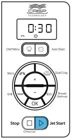
This function allows to start the Microwave function at maximum power for 30 seconds, simply pressing the Jet Start button. It is suggested for quick reheating of food with a high water content such as clear soups, coffee or tea.
